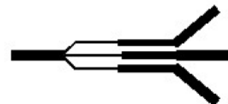
Figure .4 Layout of three-way two-stage power divider on RT/ Duroid 3010 substrate (Dim100mmX45mm)
